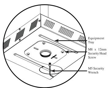
Step 1. Remove the lower mounting plate from the equipment tray by removing the four (4) M8 x 12mm security head screws with an M5 security wrench.
